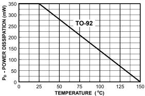
Figure 6. Power Dissipation vs Ambient Temperature
