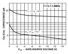
Figure 4. Capacitance vs Voltage
