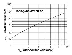
Figure 1. Transfer Characteristics
