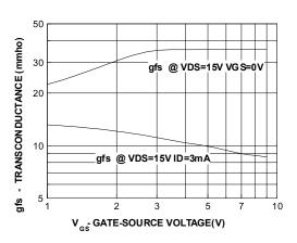
Figure 3. Transfer Characteristics
