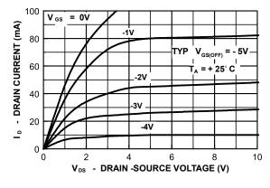
Figure 5. Common Drain-Source Characteristics
